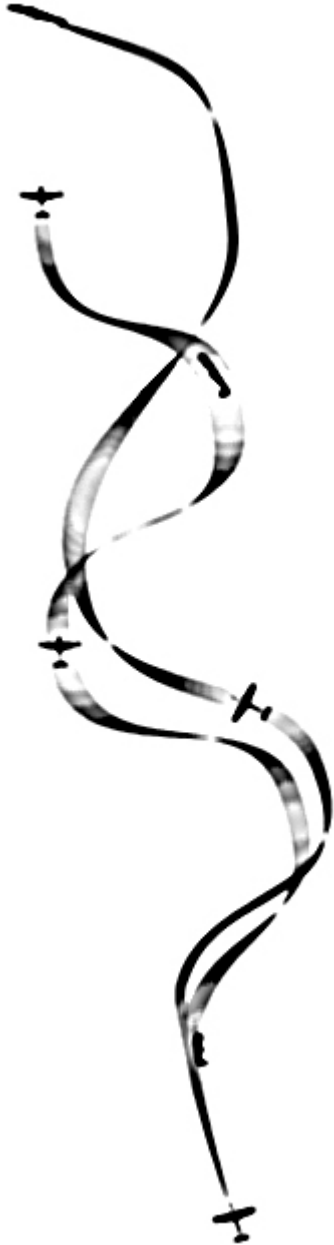
Fig 30. Flat Scissors (top view).
