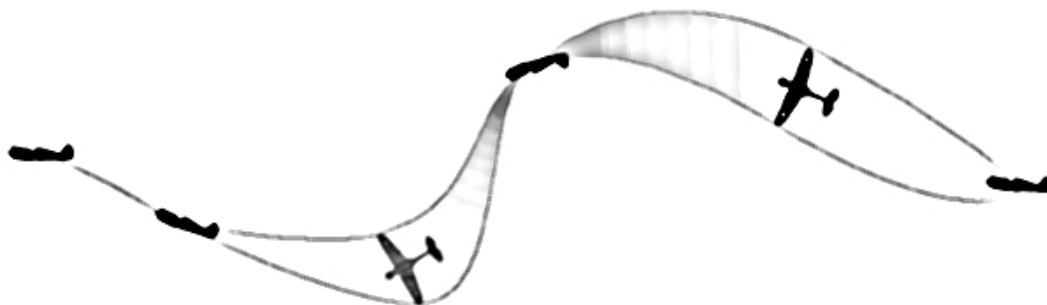
Fig 8. Barrel roll.
